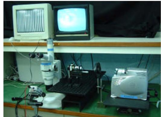
Figure 2 Hardware setup of the developed micro-level measurement system
